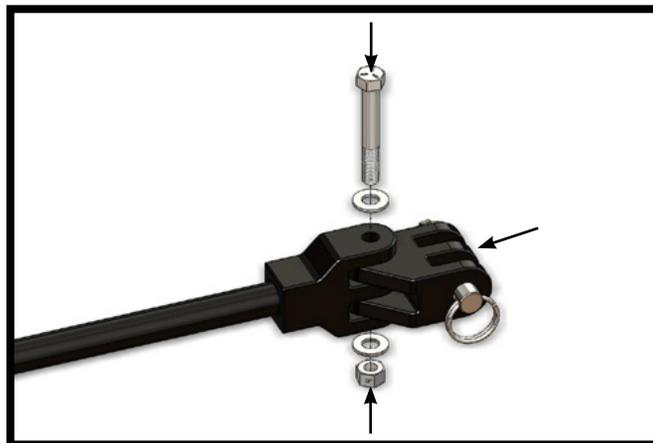
1. Install the lug onto the tow bar leg with the 1/2"-13 x 3-1/2" bolt, 1/2" washers and 1/2"-13 lock nut provided. Do this on both tow bar legs.
